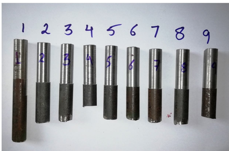
Fig. 2: Plain Turning machined Specimens
