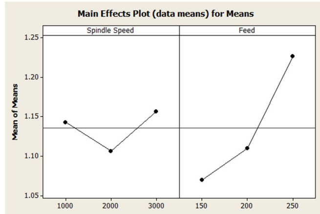
Fig. 3: Main effect plot for Delamination Factor
