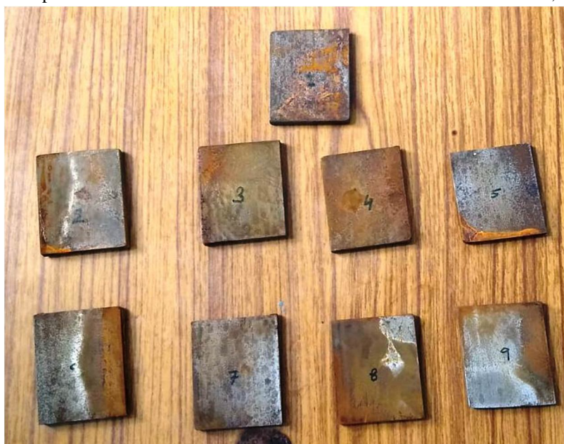
Fig. 1: AISI 1018 Specimens after corrosion test
