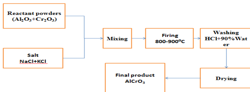
Fig.1 molten salt synthesis flow chart
