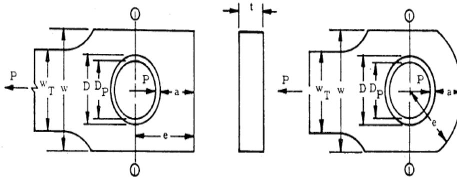
Fig 4 : Schematics of lugs loaded in tension
