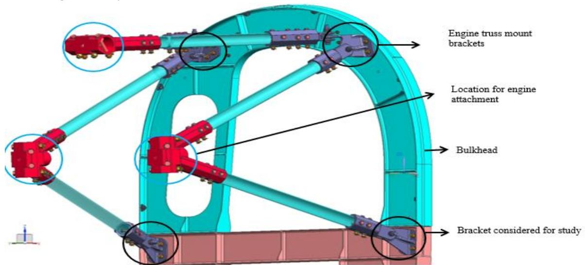
Fig 6 : Truss Structure
