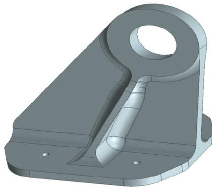
Fig 1: Engine Truss Mount Bracket
