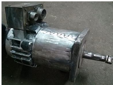
Fig 1 Photograph of PMDC Motor
