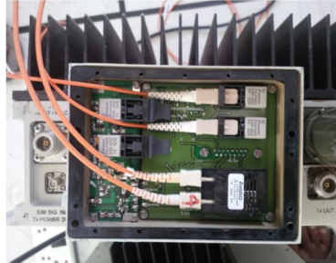
Fig4: Fiber trasmitter unit
