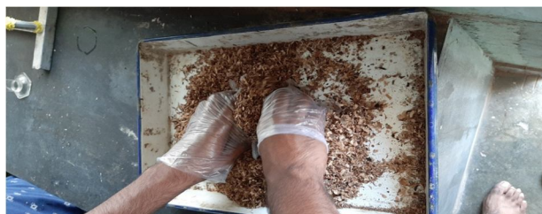
Fig.1 (b) Mixing of sun dried teak wood saw dust with H_3PO_4
