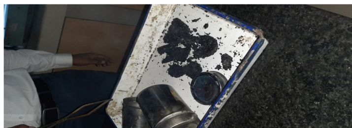
Fig.1 (c) Activated carbon obtained after burning in muffle furnace
