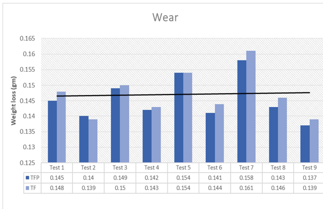
Fig. 8: Experimental conditions Vs Wear resistance at Track Diameter 70 mm, Speed 200 RPM.
