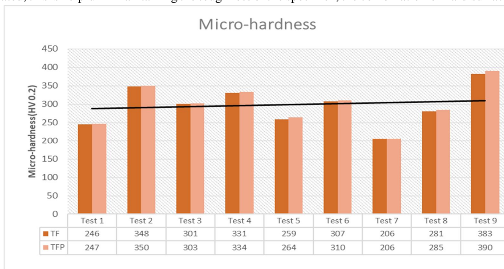
Fig. 5: Experimental conditions vs Microhardness of A105 steel at HV 0.2.
