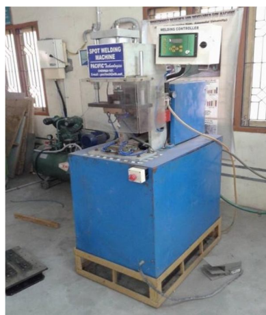
Figure 4.1 Photographic View of the ERSW machine deployed in this study
