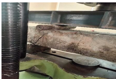
Fig. 7 flexure test on beam without SRWT mould
