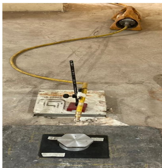
Fig.21 Radiography Testing Set-up
