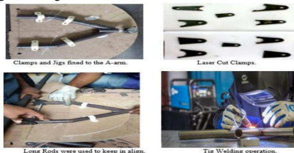
Figure 18: Setup of jigs, Fixtures for manufacturing feasibility.
