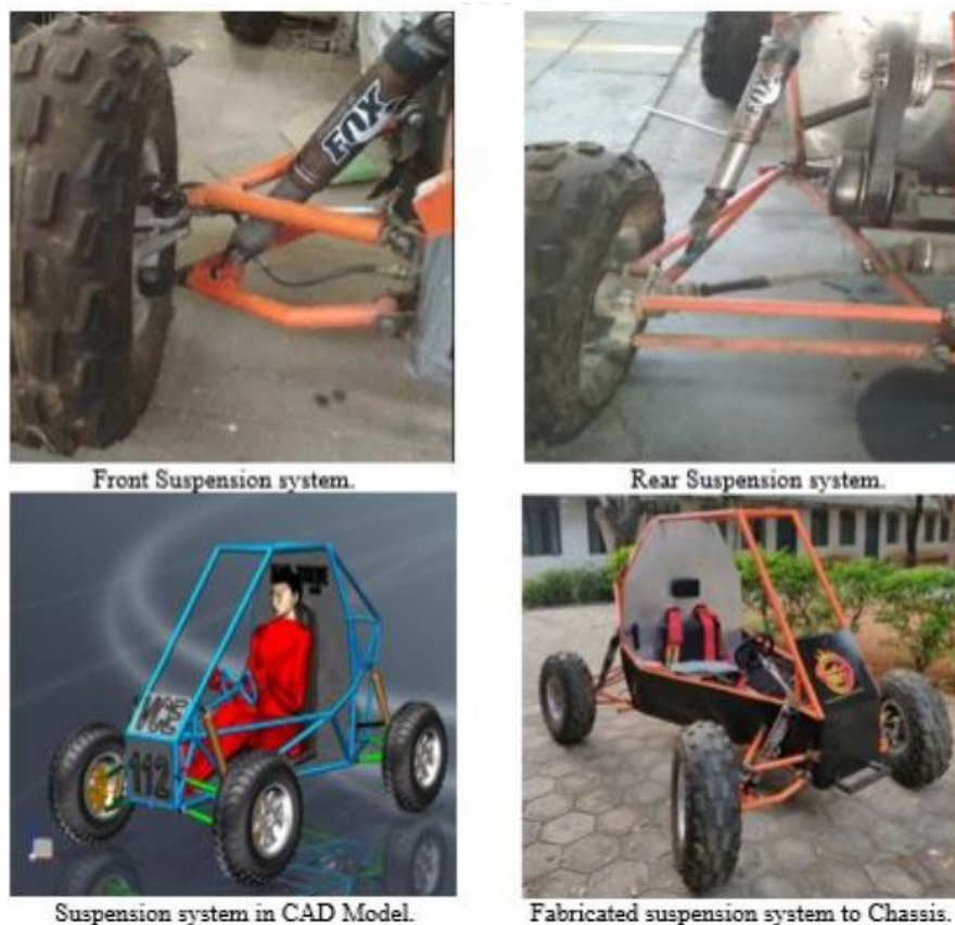
Figure 19: Assembled suspension system to the chassis.
