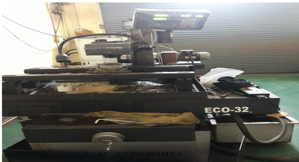
Figure.2.1 Setup Wire cut electro discharge Machine (WEDM)
