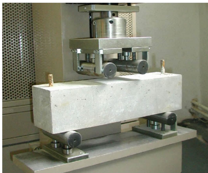
Figure 1. Flexural strength of plain cement concrete beam after testing
