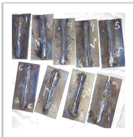
Fig.2. Weld Specimen 9 sample for L9 orthogonal Array (100mm x 60mm x 5mm)
