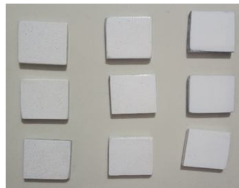
Figure 2: mild steel sample after coating
