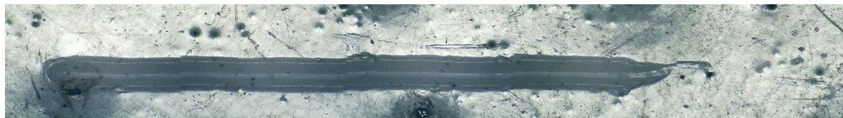
Figure 7: Scratch on the coating of 0 % reinforcement SiO 2
