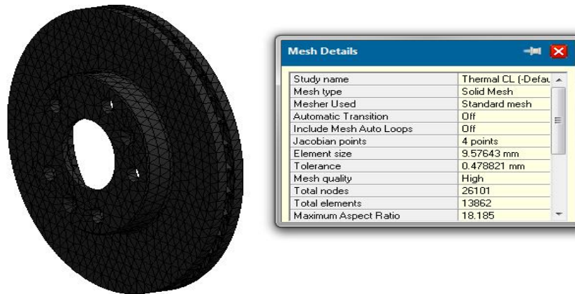
Fig. 2 The brake disc meshing
