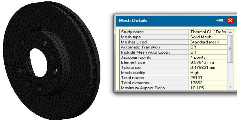
Fig. 2 The brake disc meshing
