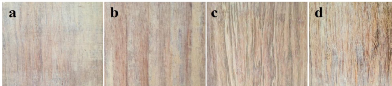
Fig 1: The surface of bamboo scrimber with different textures (a wood grain; b strip shaped; c mountain shaped; d pattern of vortices)[10]
