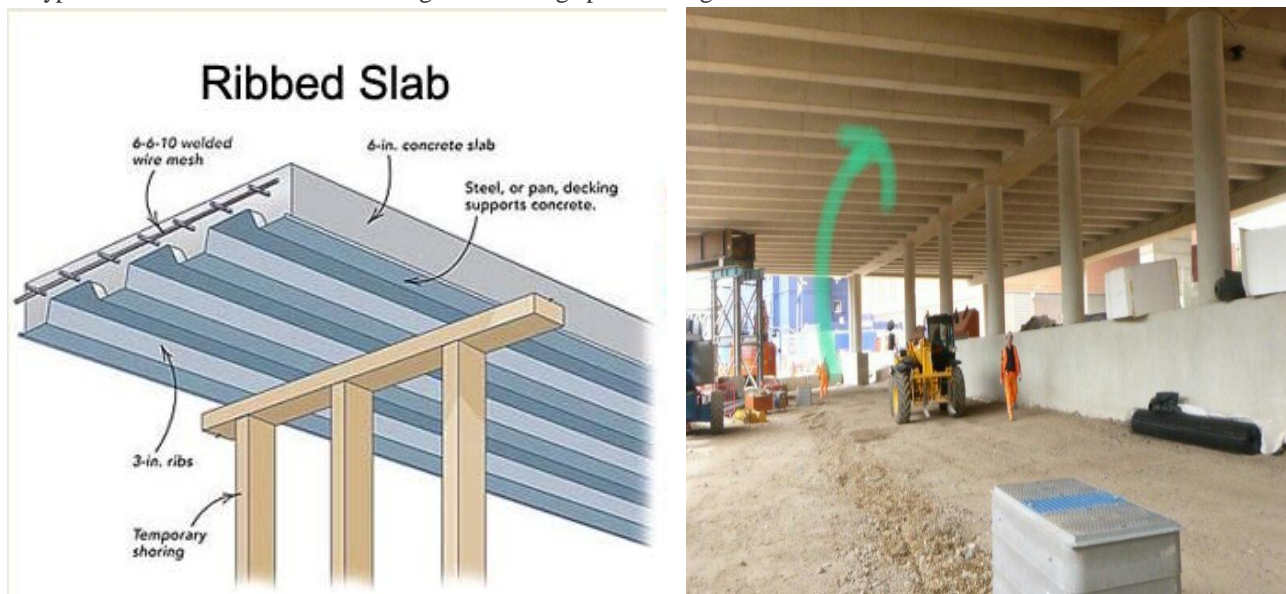
Fig. 2: Typical examples of ribbed slab
