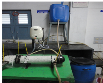
Fig. 6 Apparatus of Shell and Tube heat exchanger
