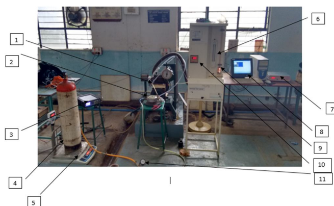
Figure II-1. Computerized 4 stroke, single cylinder petrol engine test rig
