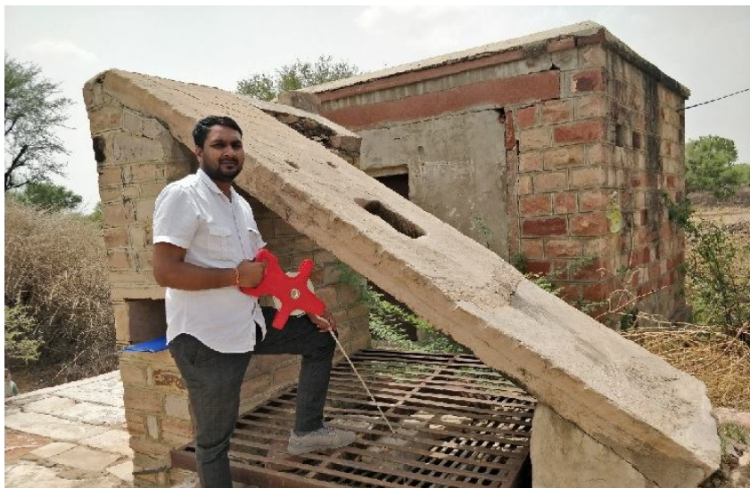
Figure 4. Measuring groundwater level of open well in degana block
