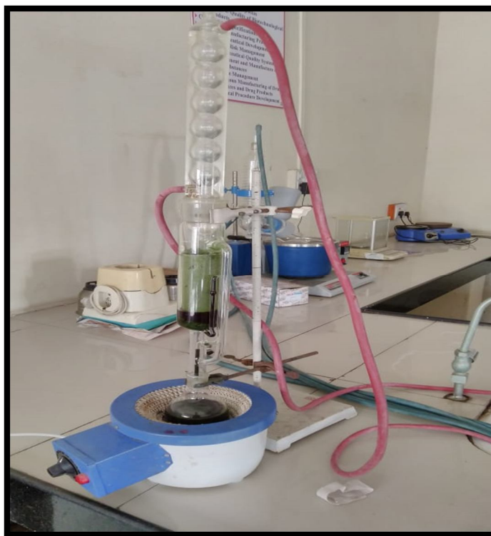
Figure No. 2: Soxhlet extraction of Cissus quadrangularis .
