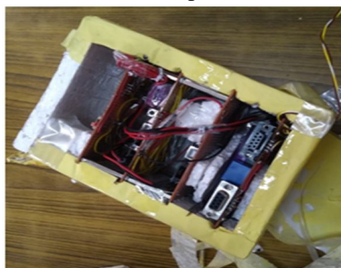
Fig 10. Cubesat Proto Model with stacked board
