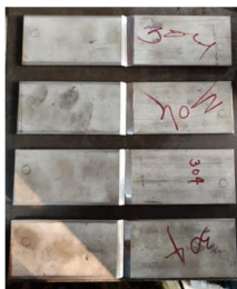
Fig 3: workpieces with single V groove
