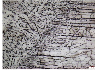
Fig 11: microstructure of SS-316L HAZ
