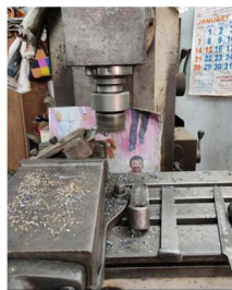
Fig 2: End milling operation on vertical milling machine
