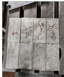
Fig 1: work pieces after removing all irregularities in length
