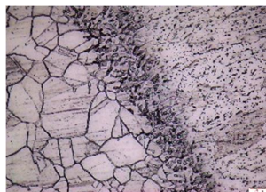
Fig 9: microstructure of SS-304 HAZ
