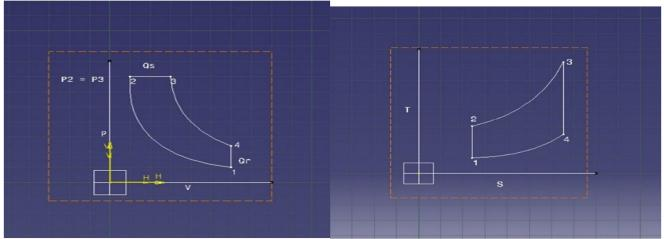
Fig 1. PV TS Diagram of Diesel Cycle.
