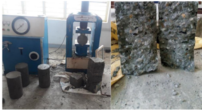
Figure 2: Split Tensile Strength setup and splitted sample
