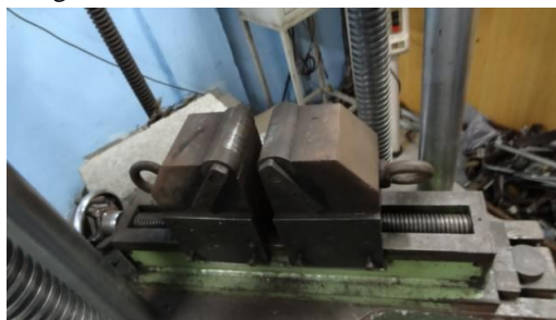
Figure 1: Attachments for bend test in UTM
