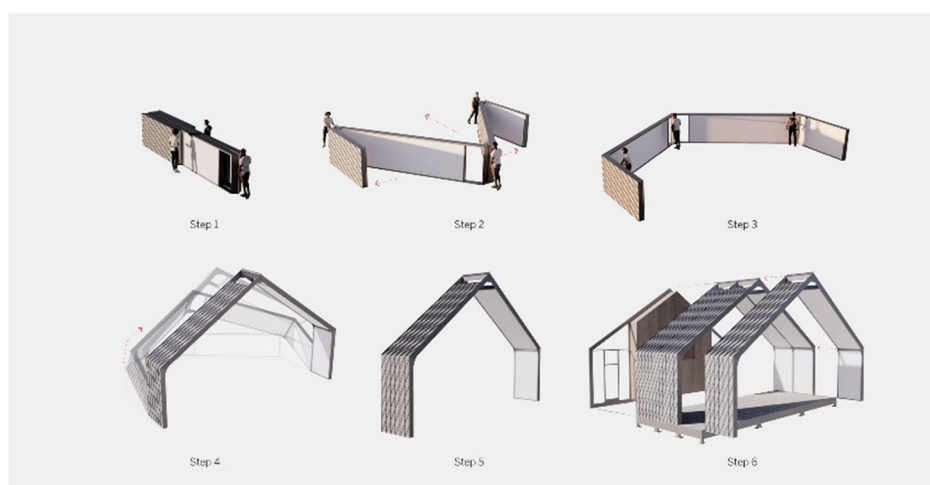
Figure 4- Construction panels design by SOM Architects (USA), (Source- (Ravenscroft, 2020)
