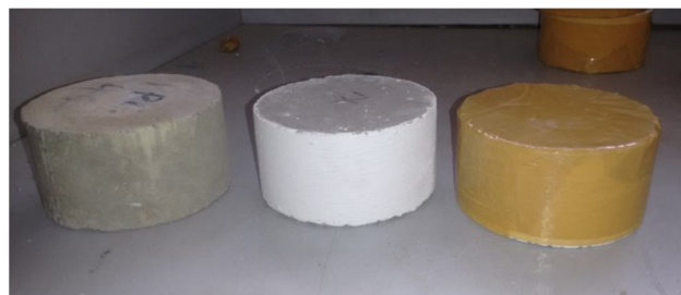
Preparation for Sorptivity test
