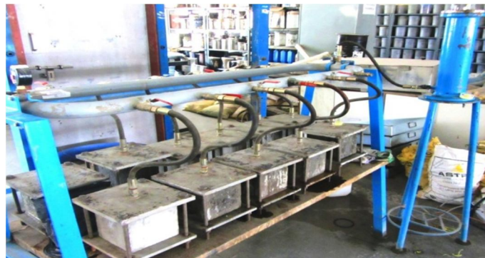
Water Permeability setup
