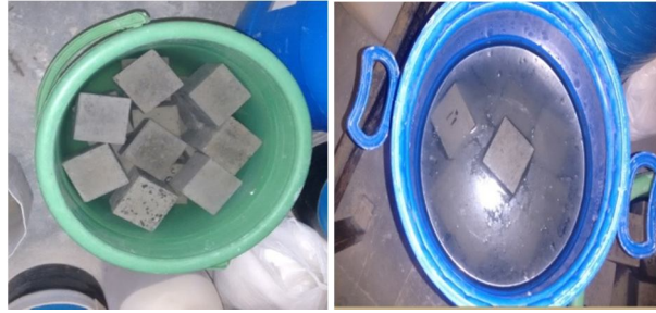
Sample placed in H_2SO_4 and Sodium Sulphate
