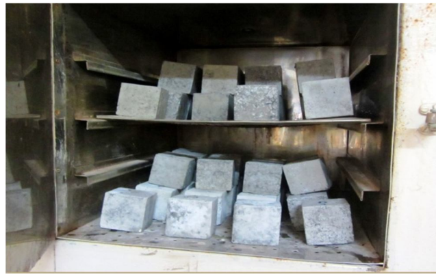
Oven curing of cubes
