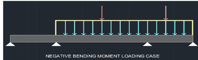
Fig. 5. Shows the loading of the deck with an eccentric uniform load which would give a negative bending moment; a hogging deck. This case shows the off-centre region of the bridge deck to have been loaded uniformly and as with the case of uniformly distributed load, here also the load acting has been considered as acting at respective proportions mid-point.
