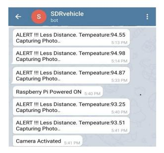
The notification of less distance and temperature value is given by the use of telegram bot SDRvehicle. It is the open source that we can gather the information and take necessary steps to avoid these type of violations.
