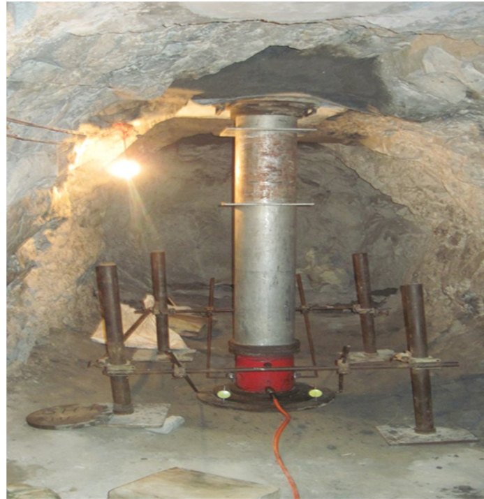
Fig. 3 In-situ Plate Load Test Setup
