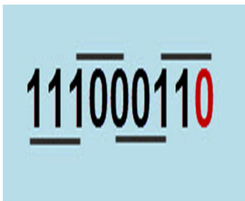
Fig. 2 3-bit pairing for Booth recoding
