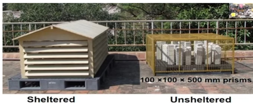
Fig 1: shows effect of carbonation in sheltered and unsheltered (open to sun)
