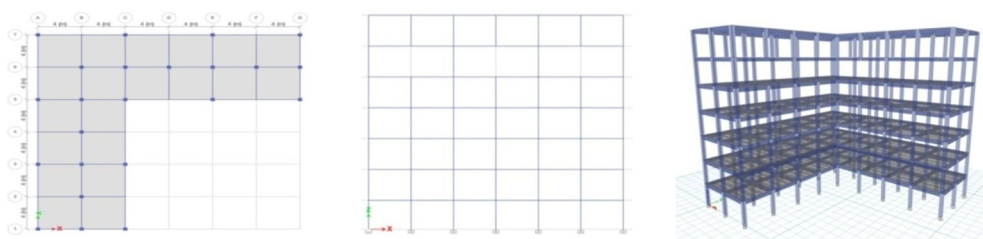
Fig.9 : Plan and section of L shape building with floating column at top corner
