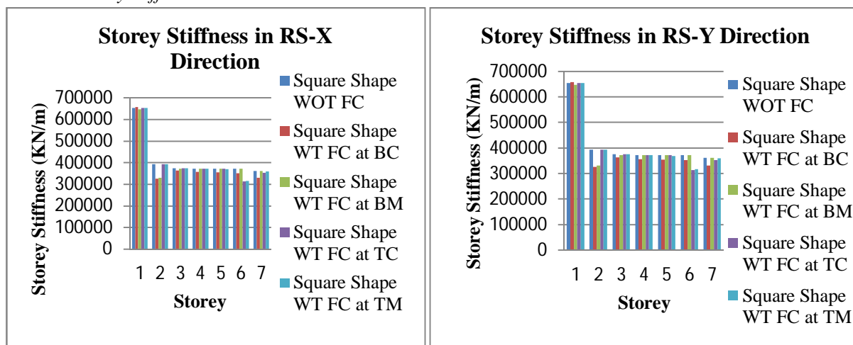
Fig.27: Square Shape Building Stiffness in RS-X & RS-Y Direction
