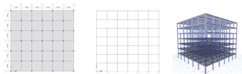
Fig.2 : Plan and section of square building with floating column at top corner
