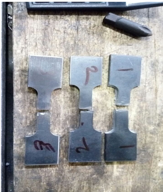
Fig.3;Dumbbell shape work pieces for tensile test
