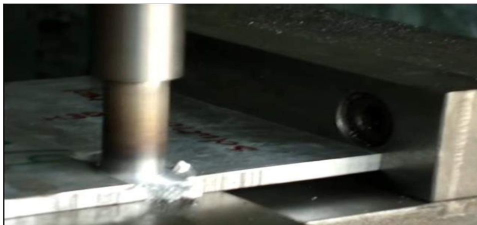
Figure 6.9: State of FSW welding after 25 seconds
