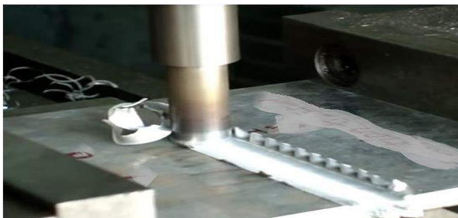
Figure 6.13: State of FSW welding after 205 seconds
