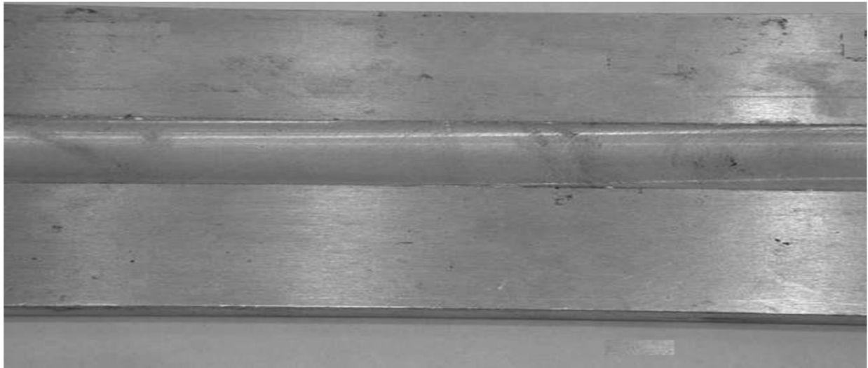
Figure 6.4: Friction stir welding product of figure 6.1 (c)
