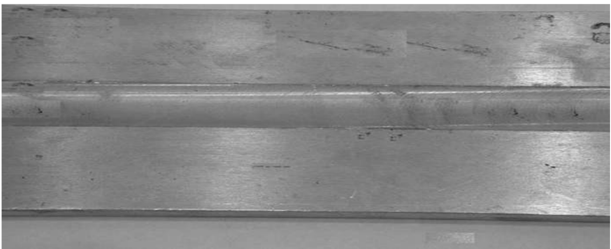
Figure 6.3: Friction stir welding product of figure 6.1 (b)
