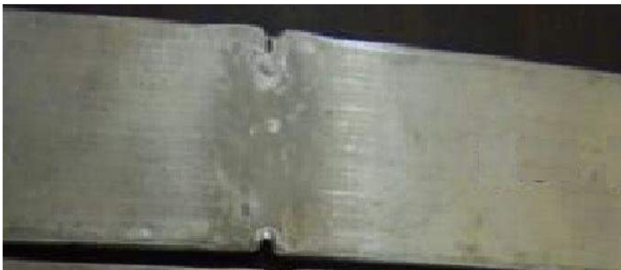
Figure 6.6: Friction stir welding product of AA6061-O and AA6061-T4 of first pair
