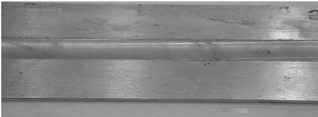
Figure 6.2: Friction stir welding product of figure 6.1 (a)
