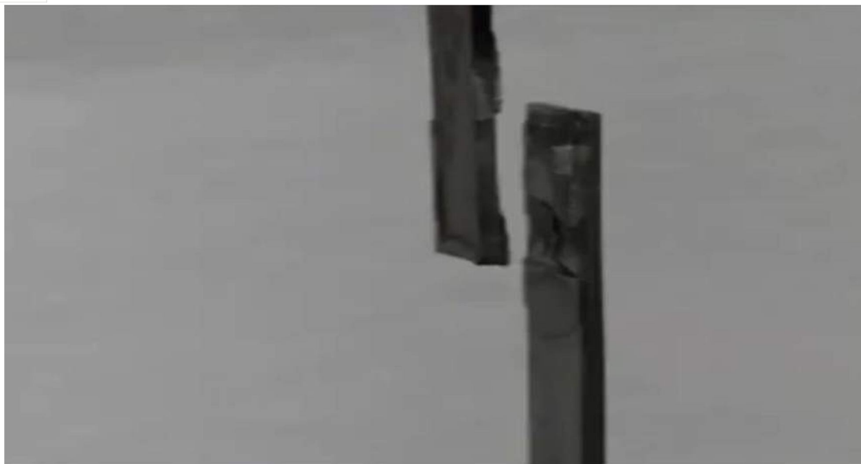
Figure 6.15: Failure of the single lap joint preparation after applying tensile stress Figure 6.15 is showing the final failure of the joint.
