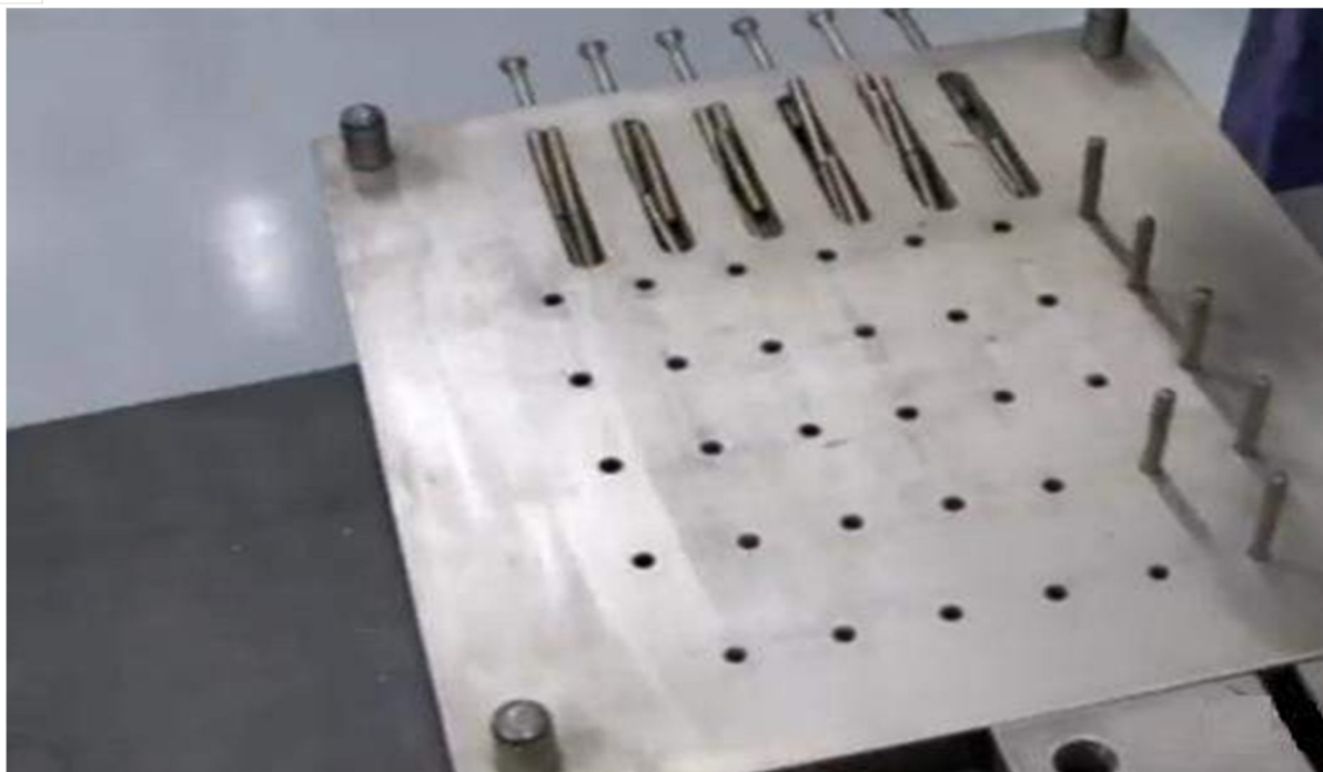
Figure 6.5: Single lap joint preparation setup
