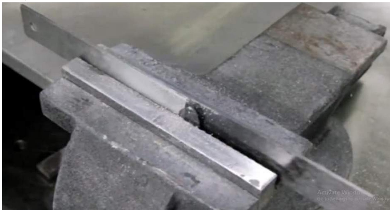
Figure 6.9: Removing unwanted material from single lap joint preparation
