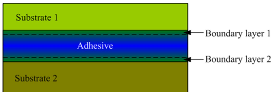
Figure 1.2: Structure of adhesive joint [40]
