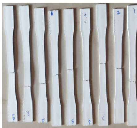
Fig. 6 Injection molding test specimen after testing
