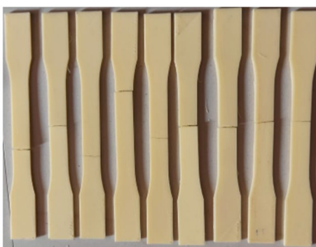
Fig. 4 3D printed specimen after testing
