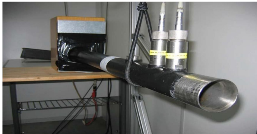
Figure 5-1 Test Set-up for reflection coefficient measurement at an open end
