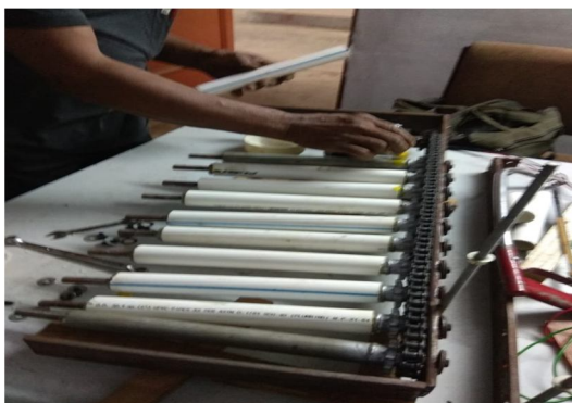
Fig-7: Figure showing assembly of rollers
