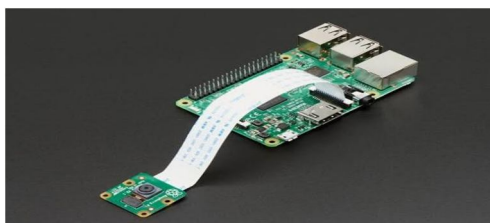
Fig 1. Raspberry Pi with Pi Camera Attached.
