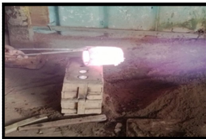
Figure: A Sample Piece heating at 700 0 C
