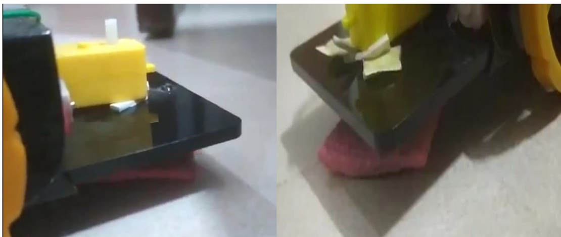
Figure 5: Floor cleaning mechanism
