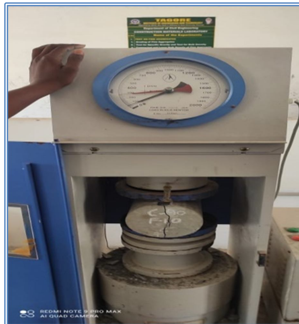
Fig.2. Split tensile strength test of cylinder specimen
