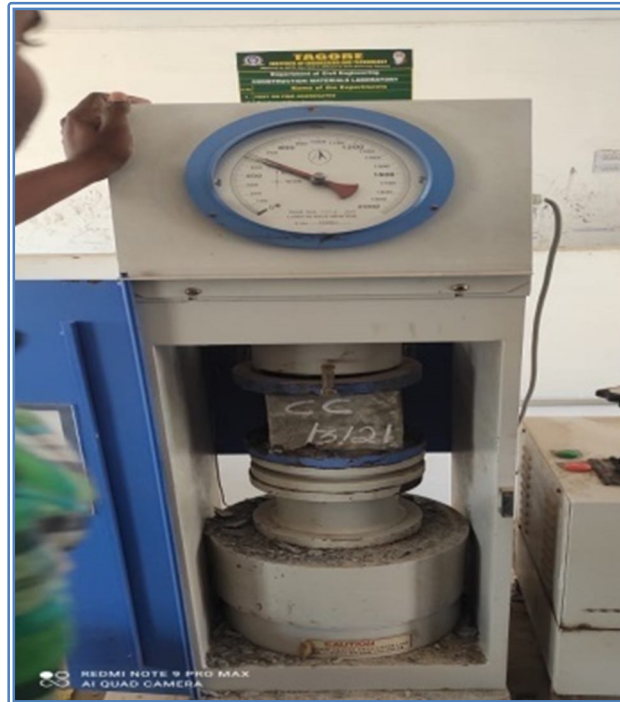
Fig.1. Compressive strength test of cube specimen
