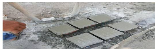
Fig-4 Casting of cubes
