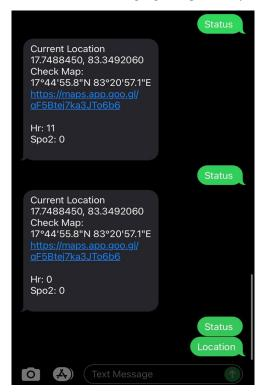
If the person removes the device then we see that the hr and spo2 values fall to zero and it's the same when the person gets in touch with the device as it takes few seconds to get right values.
