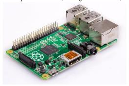
The Raspberry Pi has no built-in room. The Raspberry Pi's operating system is mounted on an SD card with a storage capacity ranging from 8 to 64GB. It has 40 pins overall, with 26 of them being GPIO pins (General purpose input/output)
