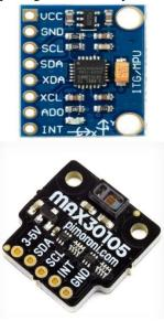
The MAX30105 is a biosensor with pulse oximetry and heartbeat monitoring built in. Photodetectors, internal LEDs, and optical modules, all of this, as well as low-noise electronics and ambient light rejection, is included in the kit. The MAX30105 is a full framework solution that makes design-in for smartphone and wearable devices even easier.
