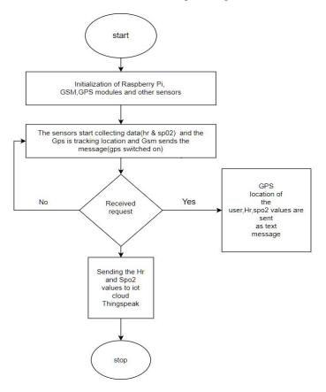
When the prototype first begins, the raspberry pi, GSM, and Gps modules, as well as other sensors, are initialized, and then they begin gathering data. The Gps keeps track of the user, and when the Gsm module is ready, it sends a notification to the phone. If anyone requests the device, it sends the sensor values along with the Gps position to the assigned phone number, and the sensor values continue to update in the Iot cloud Thingspeak, where the data is plotted and can be displayed later.
