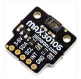
The MAX30105 is a biosensor with pulse oximetry and heartbeat monitoring built in. Photodetectors, internal LEDs, and optical modules, all of this, as well as low-noise electronics and ambient light rejection, is included in the kit. The MAX30105 is a full framework solution that makes design-in for smartphone and wearable devices even easier.
