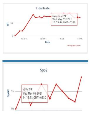
We observe that the X-axis on both the graphs is time and y-axis is Heartrate and Sp02. We see that starting 6-7 seconds heartbeat is showing garbage values and after that it starts showing correct values and we can see that for every 2 seconds the values are getting entered.
